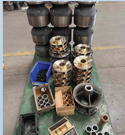
Components of a Model J11HC 11 Stage NSF certified pump ready to go to assembly. This one of several pumps, now on order, destined for a water distribution booster station located in Salt Lake City, Utah.
